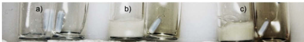
Fig. 6. Tilted samples showing cross-linked (the left of the two samples containing modified starch and KPS 2%) and not cross-linked (the right of the two samples containing native starch and KPS 2%) starch solution with concentrations 1% (a), 5% (b) and 10% (c). The small rods are magnetic bars used for creating a homogeneous mixture during the photopolymerization. However, as the viscosity increased the rods were out of use.
